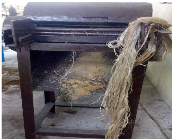
Figure 12: Pictorial Front View of the Plantain Fibre Extracting
