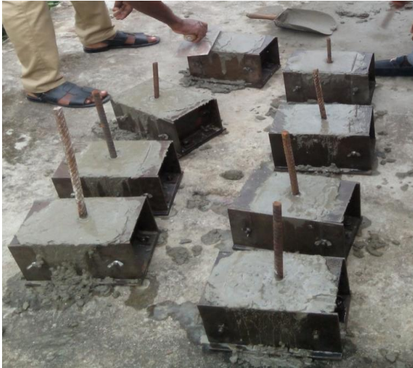
Figure 3: Placement of reinforcements into the cubes.
