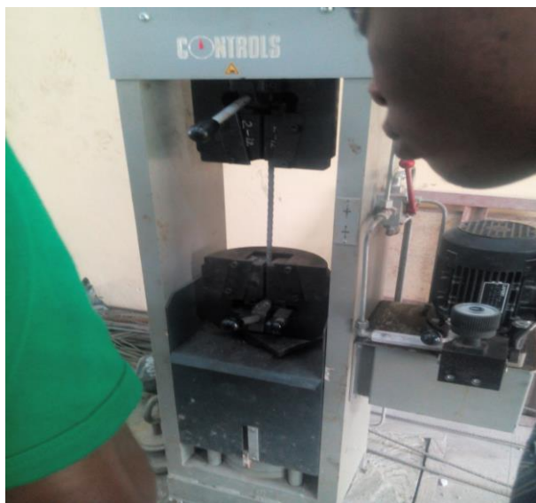
Fig. 5 Experimental set-up of the tensile test.
