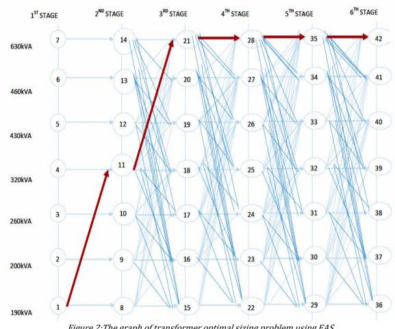
Figure 2: The graph of transformer optimal sizing problem using EAS.
