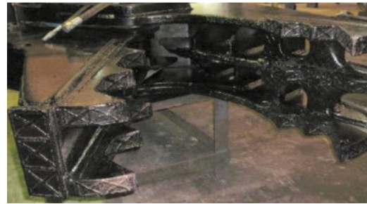
Fig. 7: Waffle hardfacing pattern [56]
