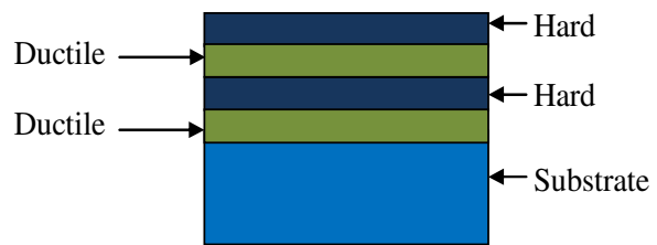
Fig. 6: Build-up of worn surface using alternate hard and ductile deposits
