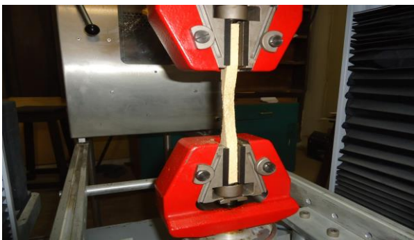
Plate II (a) Test set up for Tensile strength
