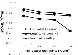
Figure 5: Hardness against moisture content
