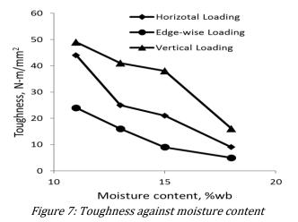
property varies from 43.75N-m/mm to 8.865N-m/mm for horizontal loading, from 23.563N-m/mm to 5.370N-mm/mm for edge-wise loading and from  $44.667\pm11.87$  to  $16.349\pm6.91$  N-m/mm for vertical loading respectively. The effect of moisture on toughness can easily be seen on the graph.
