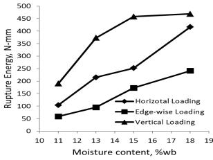
Figure 6: Rupture energy against moisture content
