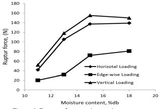
Figure 4: Rupture force against moisture content
