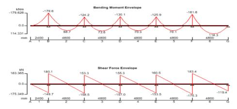
Fig 8: Bending Moment and Shear Force Envelop (Eurocode 2)
