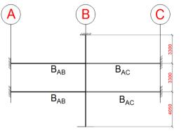
Fig. 7: Sub frame sketch for Column C1
