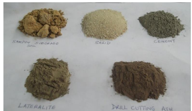
Figure 2: Soil sample, additives and binder used
