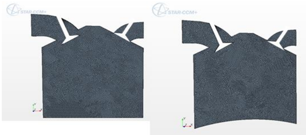
Figure 4: Infinitesimal mesh for both piston models
