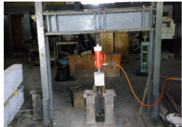
Plate 6: Pull out test set up
