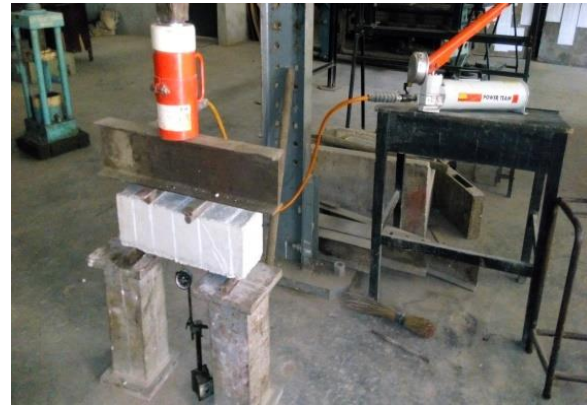
Plate 5: Flexural strength test set up.
