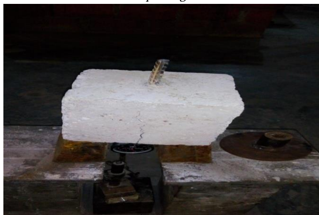
Plate 8: Pull out failure
