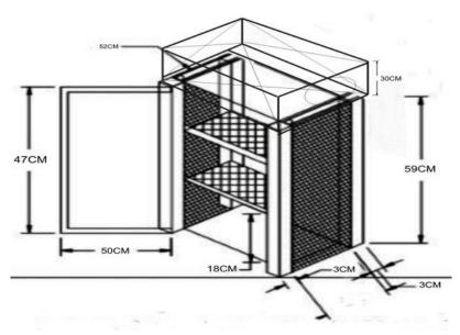
Figure 2: Isometrc view of the evaporative cooler
