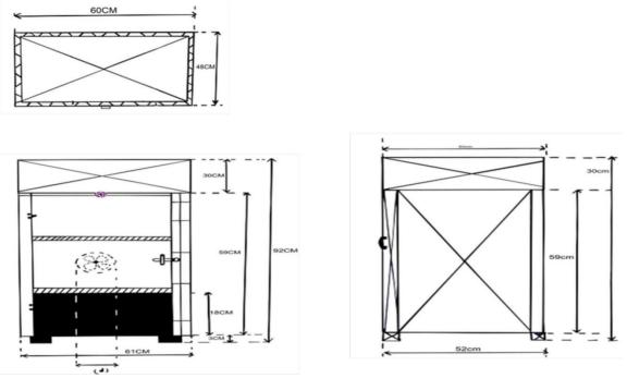
Figure 3: Orthographic view of the evaporative cooler
