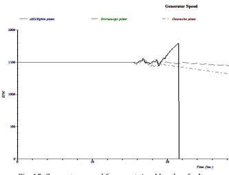
Fig. 15. Generator speed for a sustained bus bar fault
