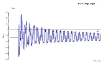
*Fig. 5. Ikeja-West bus voltage angle after line fault*
