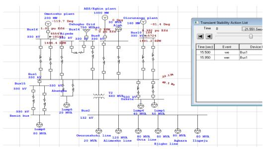
Fig. 14. Instant at which generators just lost synchronism for a sustained bus bar fault
