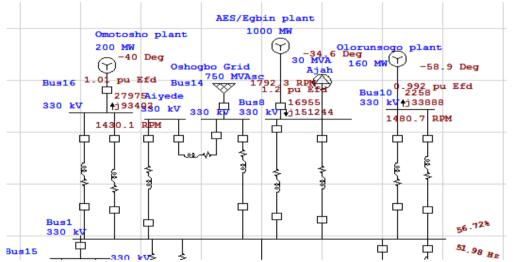
Fig. 13. Instant at which the generators is about to lose synchronism for a sustained bus bar fault
