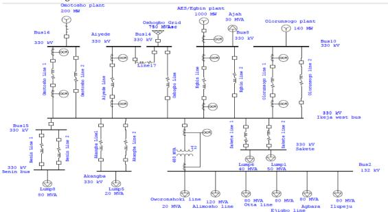
Fig.1. Single Line Diagram of the IKEJA-WEST sub-network
