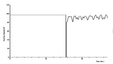
*Fig. 11. Bus voltage per hertz after a transient fault on the lkeja-West bus*
