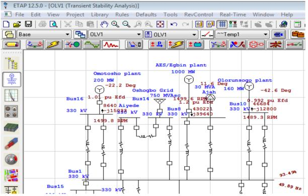
Fig. 10 Fault event simulated for a bus bar fault at Ikeja-West
