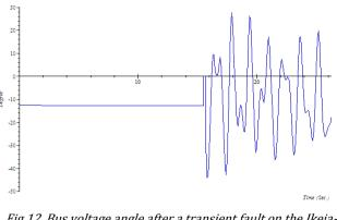
*Fig 12. Bus voltage angle after a transient fault on the Ikeja-West bus*
