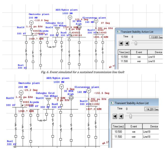
Fig. 7. Period of loss of synchronism for a sustained line fault
