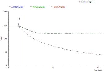
*Fig. 8 Loss of synchronism by generator after a sustained line fault*
