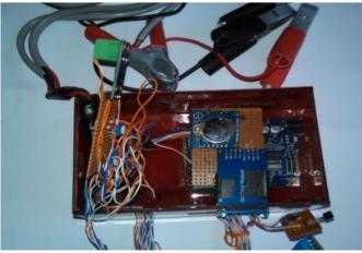
Fig. 3: Developed PV Monitoring System Prototype
