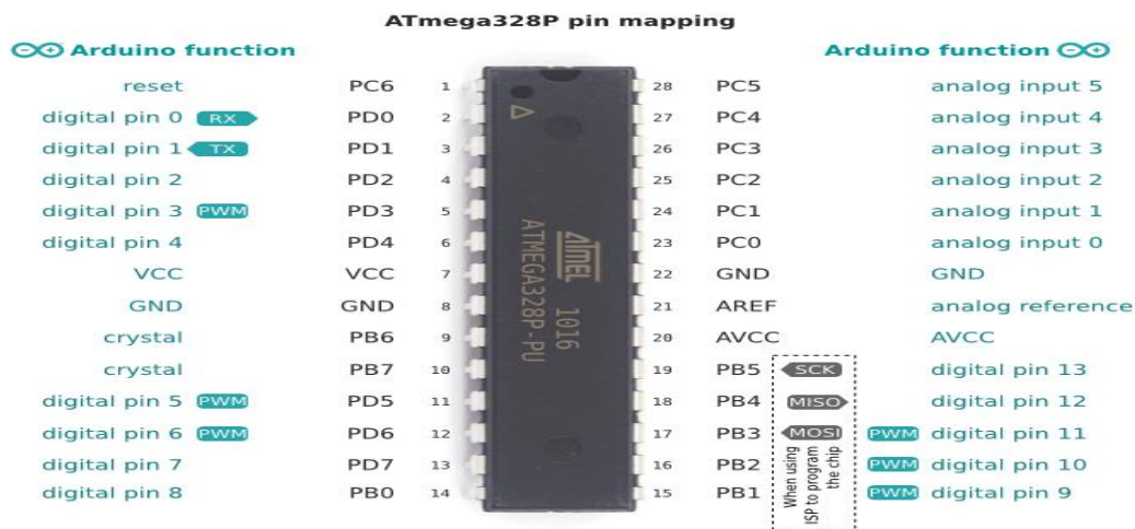
Fig 3: Pin Configuration of ATMEGA 328P PU
