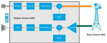
Fig. 1. A simplified cellular network transmission [11]
