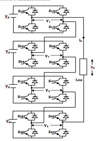
Figure 1: Configuration of 9-level cascade H-bridge multilevel inverter.
