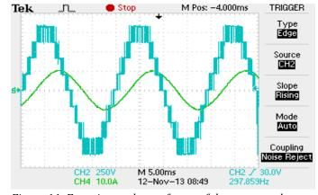
Figuer 11: Experimental waveforms of the output voltage and load current
