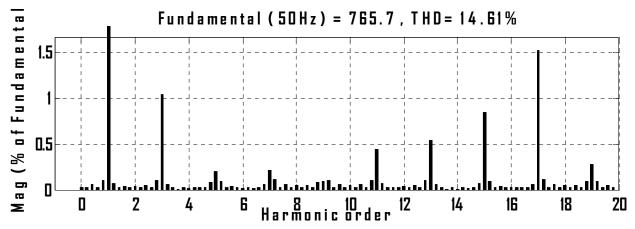
Figure 8: Harmonic profile of the CHB inverter output voltage.
