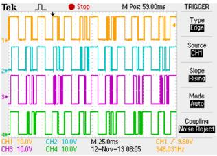
Figure 9: Experimental Gate signals.
