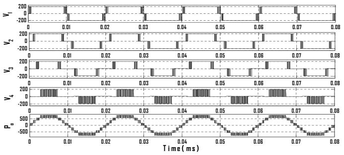
Figure 2: Voltage profile f the 9-level CHB inverter with the conventional design
