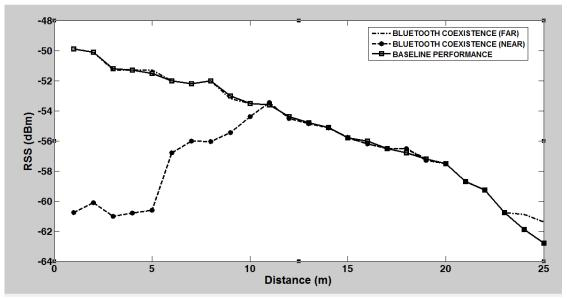
Figure 3: Comparison of Baseline Performance with Bluetooth Coexistence (RSS vs. Distance)
