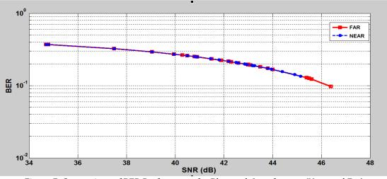
Figure 7: Comparison of BER Performance for Bluetooth Interference (Near and Far)
