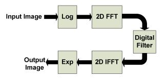
Figure 1. Frequency Domain Homomorphic Filtering Technique
