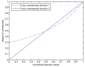
Figure 5. Mapping of logarithmic values of intensity values to fuzzy domain using fuzzy Membership Functions 1 and 2
