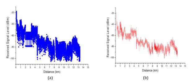
Figure 3: RSL with pick peak, (a) before filtering, (b) after filtering
