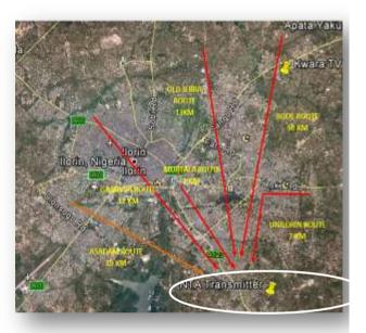
(a) (b) Figure 1: (a) Measurement routes for NTA, (b) Measurement routes for KWTV
