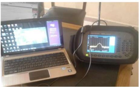
Figure 2: Agilent Spectrum Analyzer 100 MHz-7 GHz
