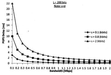
Figure 7: Delay [ms] versus bandwidth [Mbps] for only PGPS technique
