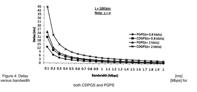
Both figures 3 and 4 show that with increase in transmission bandwidth the exponential decay in the delay is more in PGPS technique than in CDGPS. Therefore, PGPS exhibits better delay performance than CDGPS technique. In order words, results show that for a
