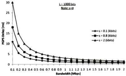
Figure 9: Delay [ms] versus bandwidth [Mbps] for only PGPS technique
