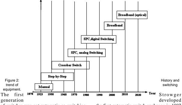
of switches was not automatic so switching was done manually using a switchboard.
