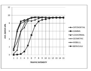
and only behaved like the other distributions when the traffic intensity increased to twelve. At low traffic intensities the behaviour of the distributions varies while at high traffic intensities they behave alike. Therefore, it is shown that Gamma distribution has the lowest buffer occupancy and delay, while Geometric and Bernoulli have the highest occupancy and delay. Figure 4: Average Waiting (Delay) versus Traffic Intensity
