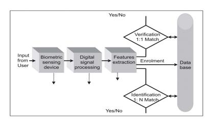
Fig 1: Diagram of Automated Biometric Systems
