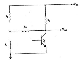
Fig.6: Equivalent circuit of the Schmitt trigger
