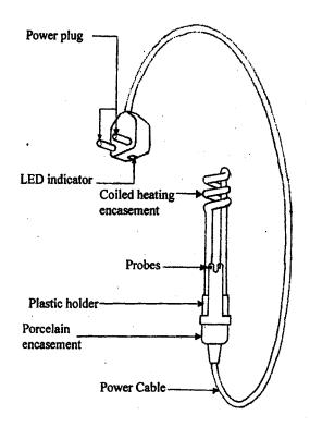
Fig 8. Water heater with safety control unit.
