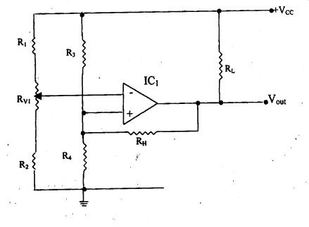
Fig.5: The Schmitt trigger
