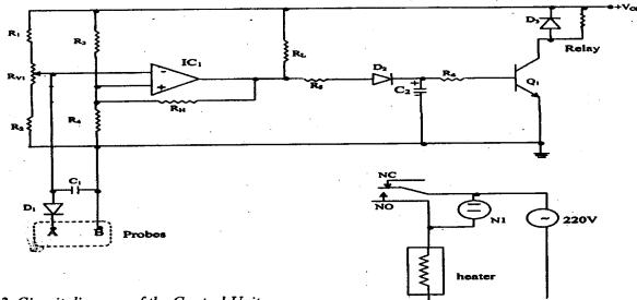
Fig. 3. Circuit diagram of the Control Unit.
