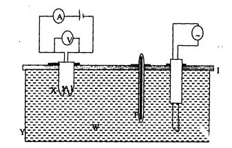
**Fig.4** Scheme for measurement of Conductance of water
