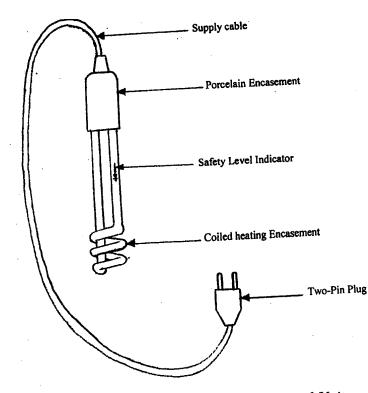
Fig.1: Heater without control Unit
