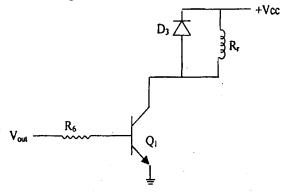
Fig. 7: Relay Driver network.
