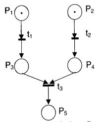
Fig. 1(a): A marked Petri net diagram (before firing)
