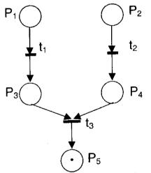
Figure 1(b): A marked Petri net (after firing)
