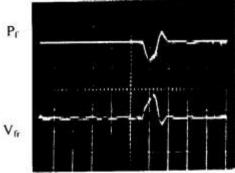
Fig. 5: Hybrid Modulation: Illustrative Steady State and Transient Waveforms under Step Change in Tank Load Resistance and Inductance {0.46 + j4.6 to 0.33 + j3.3)Ω at constant tank load Power of 480W (X<sub>Lo</sub>=3.4Ω, V<sub>s</sub>=180V, I<sub>om</sub>=2.7i<sub>op</sub>), Ct = 130µF)
