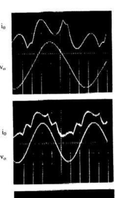
(a) Initial Steady State  $R_{to} + jX_{Lio} = (0.46+j4.6)\Omega$ ,  $\delta=160.5^{\circ}$   $f_{o} = 259Hz$  (Load current  $i_{o} - 5A/div$ , 0.5ms/div) (Load voltage  $v_{o}$ . -100V/div, 0.5ms/div)
