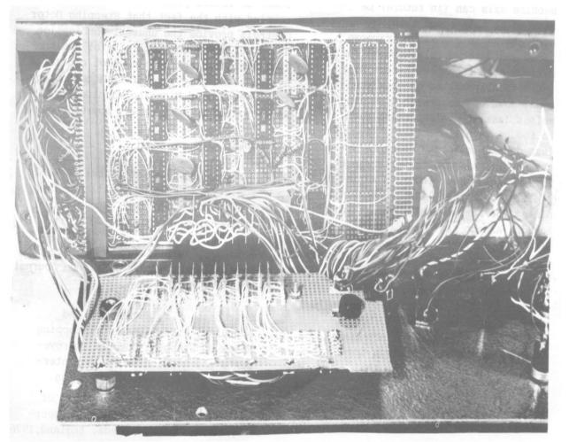
Fig. 6(b) the position command logic box and control switches the black box
