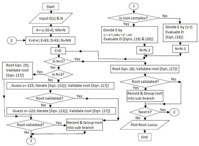
Figure 3: Flow Chart for the Determination and Plotting of Root-Locus as K Varies from 0 to ∞
