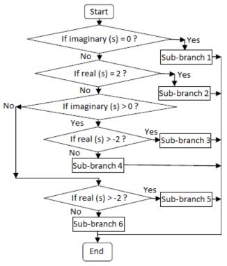
Figure 6: Flow chart for Grouping of a Root of  $G(s)H(s) = \frac{K}{s(s+4)(s^2+4s+20)}$  into a Sub-Branch.
