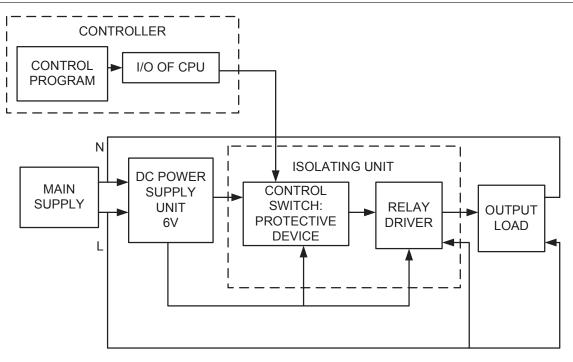
Figure 1: Block diagram of a computer control system.
