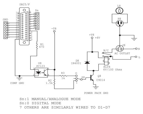
Figure 2: Circuit with optoisolation.
