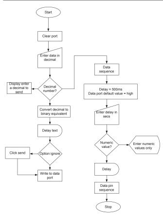
Figure 4: Flow chart for the control program.
