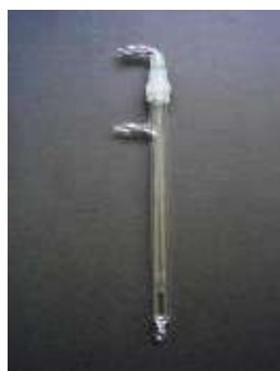
(Fig. 44) Inverted L tube and T tube combination. Water comes from the top opening and leaves from
