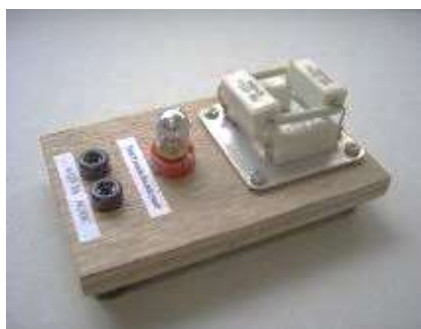
(Fig. 26) Finished mini-heater
