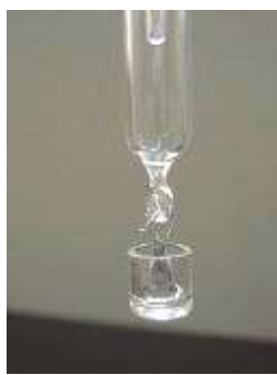
(Fig. 45) The base of the T tube has a glass ring which attaches to a small
