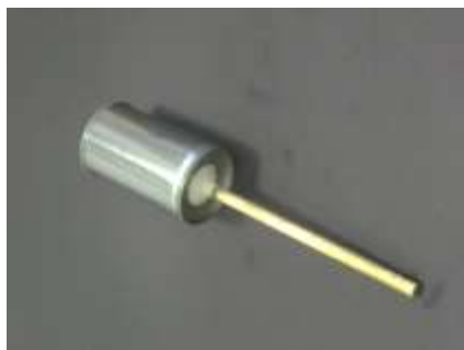
(Fig.34) Drill a central hole at the bottom of the tin, allowing a brass rod to go through. Fix by (A+B) type metallic epoxy cement.
