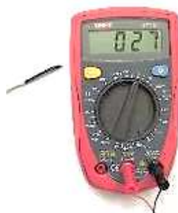
(Fig. 29) DMM with miniature thermocouple for temperature measurement
