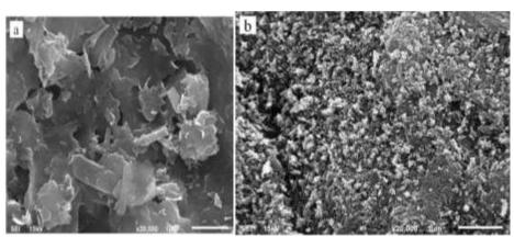
Fig (5) SEM image of a. Natural Bentonite and b. TiO2/ Bentonite composite [16].
