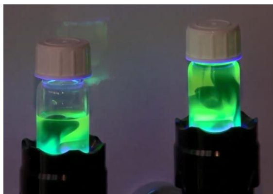
Fig. 3: Basic version of the Photo-Blue-Bottle experiments; irradiation and shaking of the PBB solution as Screenshots from video-supplements provided via Ref. [4]
