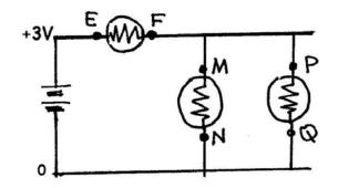
4 Figure 3 shows a circuit with bulbs of the same resistance. Predict the voltages
