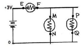
In the 35 lab reports we have as data, 82% of the students **predicted** that the potential difference,  $V_{PQ}$ , across the terminals P and Q would become zero. The **observed**  $V_{PQ}$  across P
