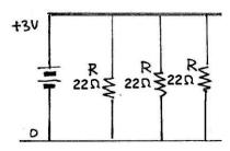
You don't have 1 ohm resistors so use the 22 ohm resistors instead.
