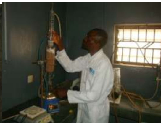
Plate 4: Oil extraction using soxhlet apparatus
