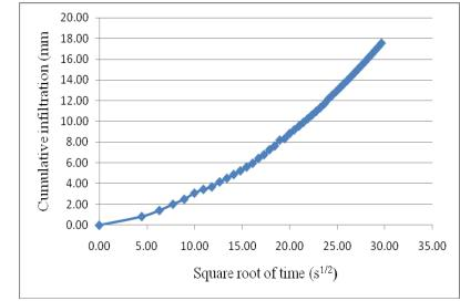
Figure 3 Cumulative infiltration versus square root of time for sorptivity in 2018
