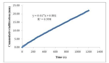
Figure 6 Cumulative infiltration versus time for infiltration rate in 2005
