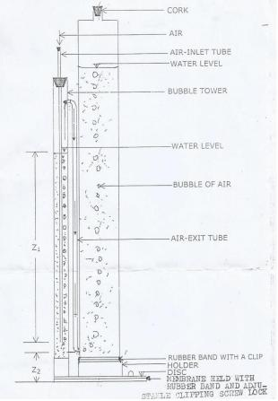
**Figure 1** A sketch of side view of the tension infiltrometer Source: Yusuf (2006)
