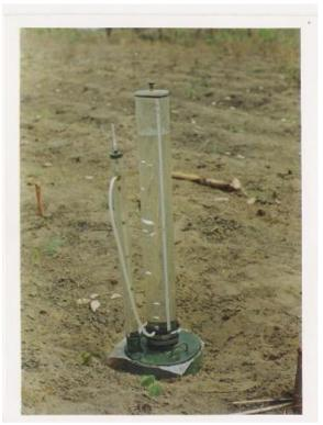
Figure 2Tension infiltrometer in operationSource:Yusuf (2006)
