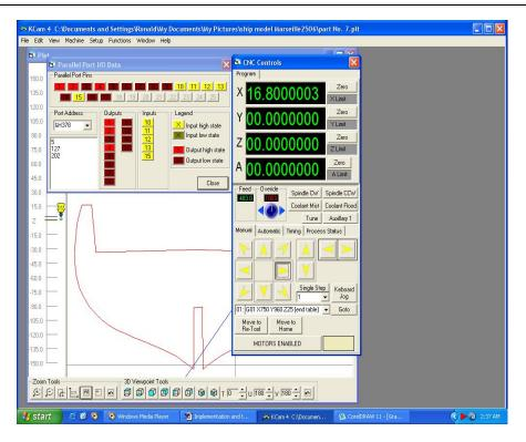
Fig 4: Parallel port testing using manual jog keys, port monitoring
