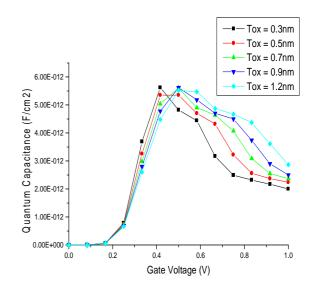
Figure 5: A graph of quantum capacitance against gate voltage for different oxide thickness in carbon nanotube MOSFET
