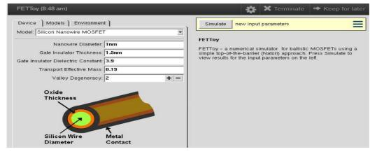
inversion condition and gate capacitance approaches the insulator capacitance. Plate 1: FETTOY Software interface
