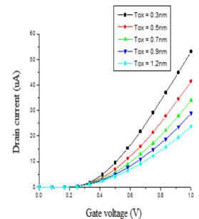
Figure 4. Graph of drain current against gate voltage for different oxide thickness in silicon nanowire MOSFET
