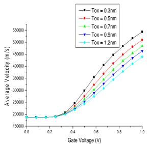
Figure 7: A graph of average velocity against gate voltage for different oxide thickness in carbon nanotube MOSFET
