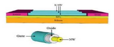
Figure 2: Silicon Nanowire Field Effect Transistor
