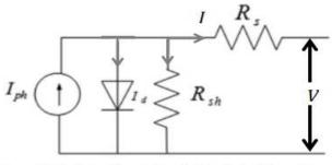
Figure 1.0: Equivalent Electrical circuit of the single diode model
