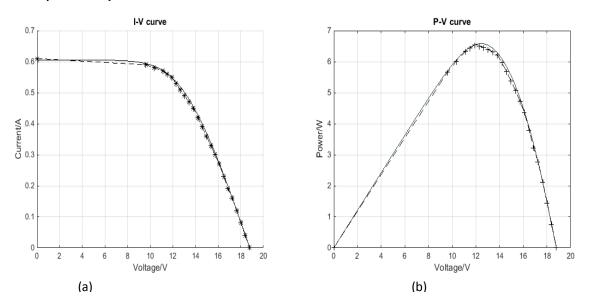
Figure 5: Characteristics curves for experimental and simulated values (a) I-V curve (b) P-V curve
