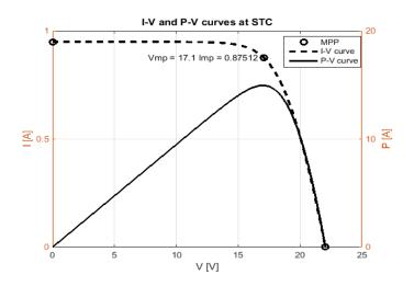
Figure 3: I-V and P-V curves at STC
