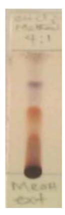
Figure 1: Chromatogram of Methanol extract developed in Chloroform:Methanol (4:1)sprayed with Anisaldehyde/  $H_2SO_{4.}$
