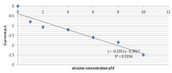
Figure 5: Calibration curve of successive additions of atrazine responses at modified electrode in 0.32 mM of atrazine solution at pH 5 at scan rate of 50 mV/s
