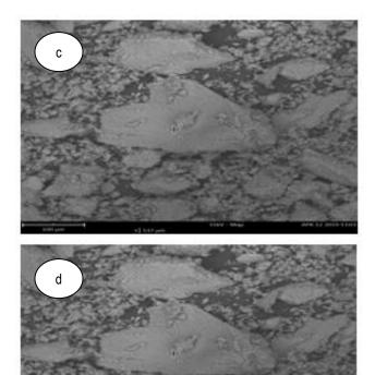
**Plate**: SEM morphology of (a) Bare Graphite Electrode (b) Graphite with Emiraldine (c) Graphite with Hkust -1 and (d) Graphite with Emiraldine and Hkust-1
