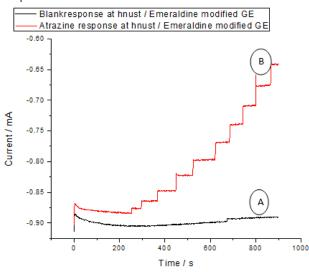
Figure 3: A- current –time response of successive additions of atrazine at modified electrode at pH 5
