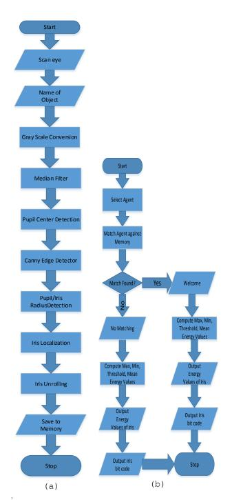
Figure 3.2: Iris acquisition and authentication enhancement flow diagram
