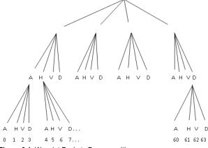
Figure 3.1: Wavelet Packets Decomposition
