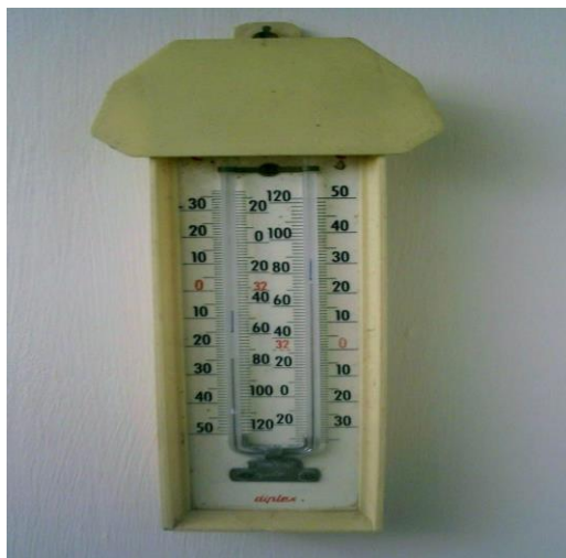
Figure 2: A Typical Outdoor Minima-Maxima Thermometer
