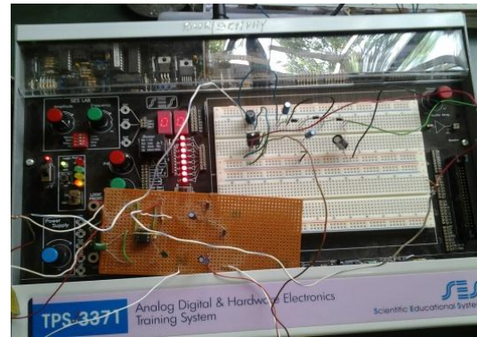
Figure 8: Prototype of the proposed high step-up dc-dc converter designed on TPS 3371.
