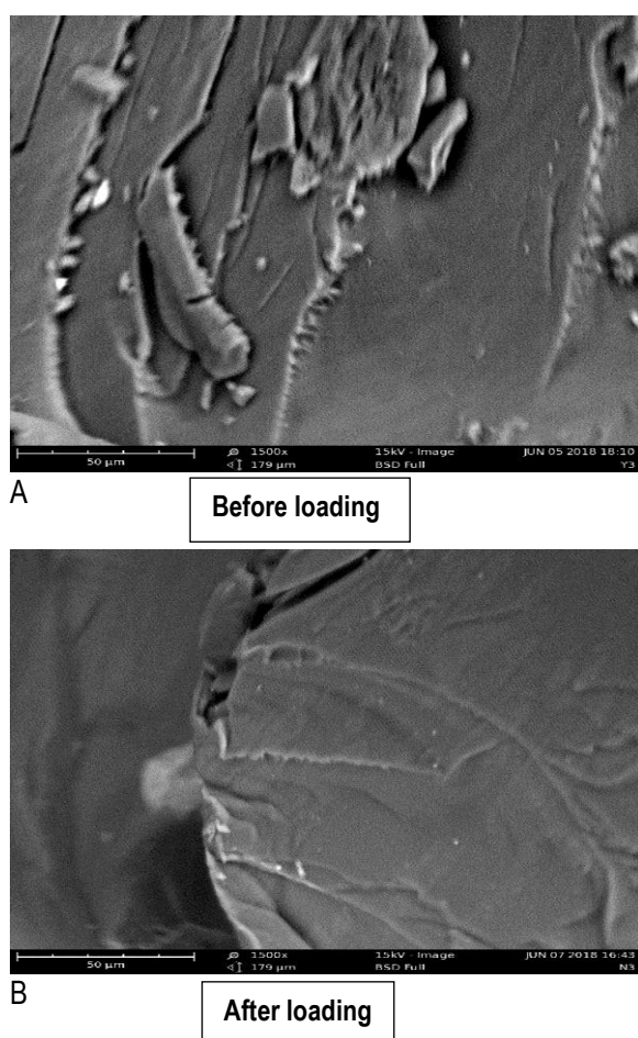
Figure 2: SEM images of S-g-Acrylamide Hydrogel Before and After Promethazine Loading
