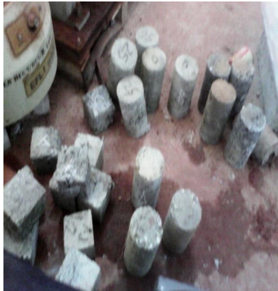
PLATE II: Cylinder concrete used for tensile strength test
