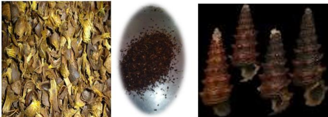
PLATE I: Palm Kernel Shell (left), crushed palm kernel shell (middle), Periwinkle Shell (right).
