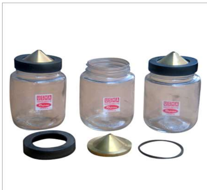
Figure 3. Pycnometer for determining specific gravity of soils.
