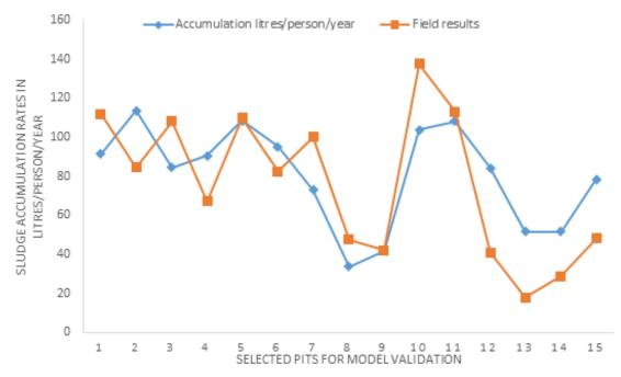
Figure 4. Comparison of simulated and experimental data.
