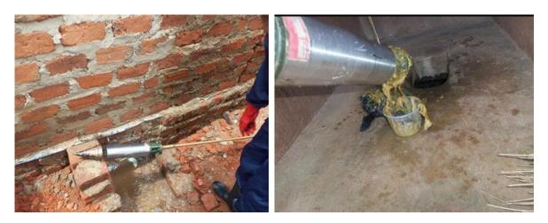
Figure 2. Sampling of faecal sludge: Pit sludge sampler (Left)-; Pit sludge sampler in action (Right).
