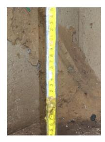
Figure 3. Depth tool with sludge markings.
