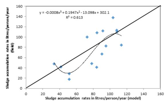
Figure 5. Simulation of model and field results showing R2 value.
