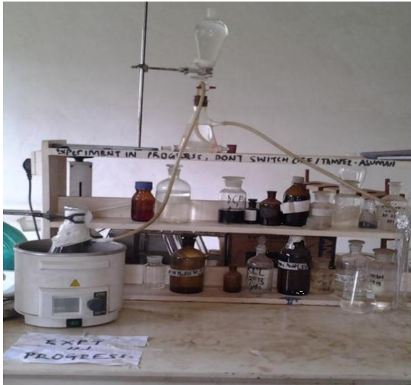
Plate 1. Laboratory experimental setup for the generation and collection of methane gas.
