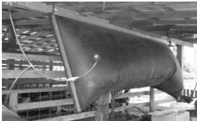
Figure 10. Flotation storage tank. Source: Forst (2002).
