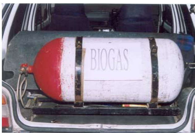
Figure 11. Biogas packed in cylinder for car consumption. Source: Vijay (2006).
