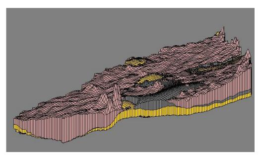
Figure 6. 3D image of the lithology of the study area created by using GMS visualization tools.
